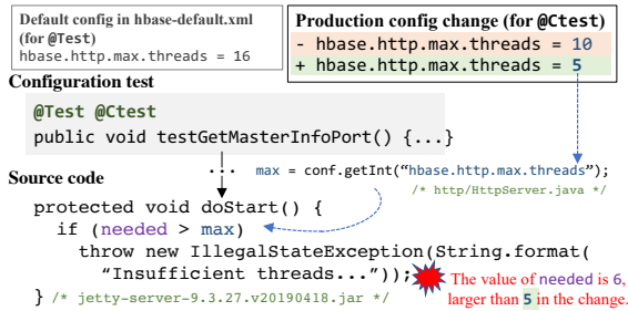
Fig. 1: A configuration test instantiated by a changed production configuration. The test fails as the code under the new production configuration throws an exception.
